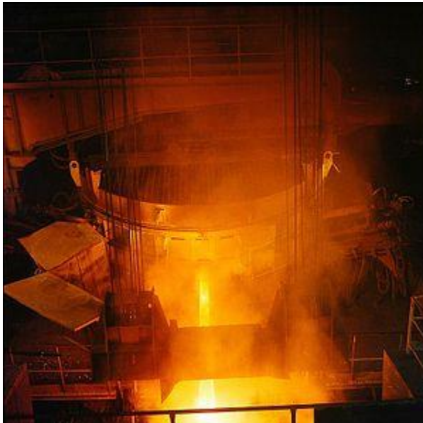
An electric arc furnace (the large cylinder) being tapped
